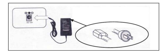
Notice: We also STRONGLY recommend that you plug the DVR and cameras into a Transient Voltage Surge Protector (UL-1449 rating). Look for a clamping voltage of 330 or lower, Joule rating of at least 400, and a response time of 10 nanoseconds or less.
